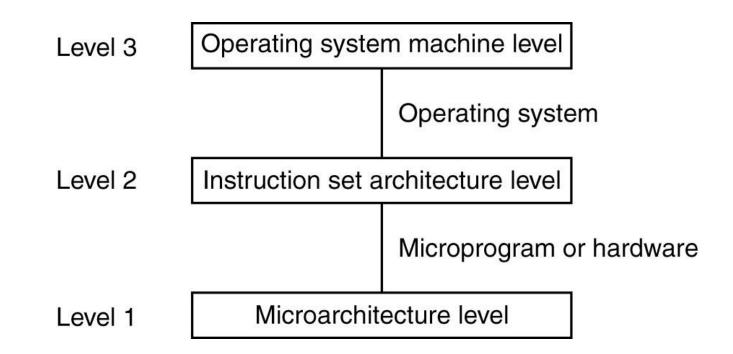
Positioning of the operating system machine level.
